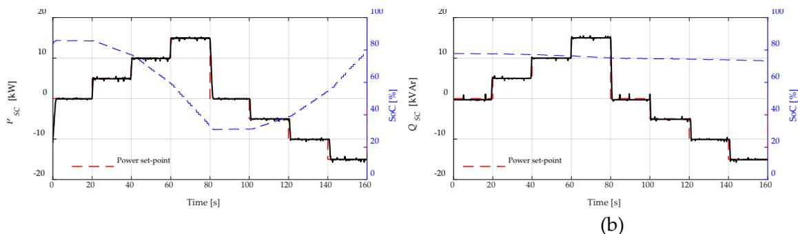
Next, regarding the response presented by the Li-Ion BESS, Figure 14 (a) shows the high effectiveness in active power setpoint tracking of the lithium-ion battery in transient and permanent regimes, shown in Figure 14 (b).
