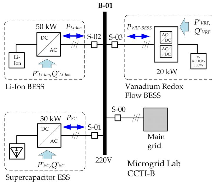
The ESSs will all be subjected to the same operating conditions to facilitate a comparative analysis between the different storage technologies. Due to the significant amount of energy handled in such tests, both the charge/discharge tests and the dynamic tests of active and reactive power set point tracking will operate one technology at a time. The following is a description of the test plan to be carried out in this study, which constitutes the methodological basis of this research:
