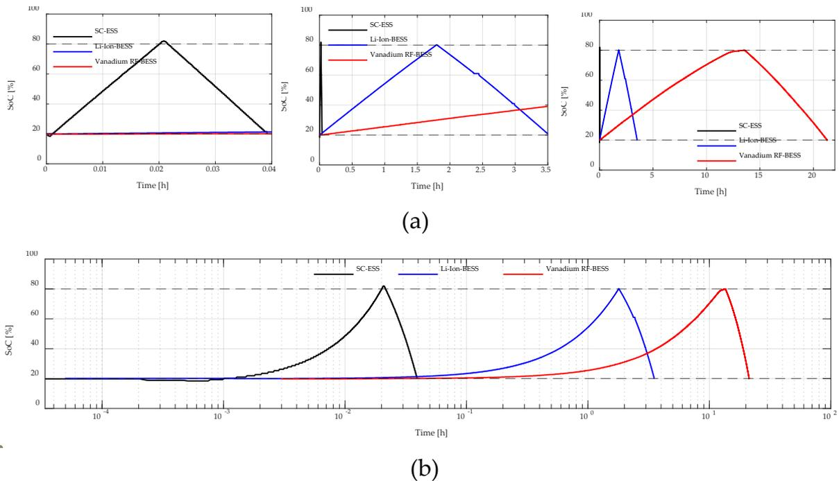
Finally, for completeness, the tests described above have been repeated to obtain the charging and discharging characteristics of the ESSs but for different power values. Table 1 shows the results obtained in the experimental tests. In each case, the round-trip efficiency becomes a characteristic value of each ESS technology and varies very little for each charging
